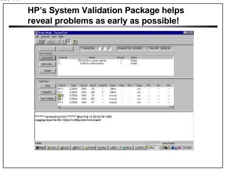
The screenshot above is from the HP E2920 family System Validation Pack (SVP), showing 2 test scenarios (top), 5 test card resources (middle) and test status report window (bottom).
