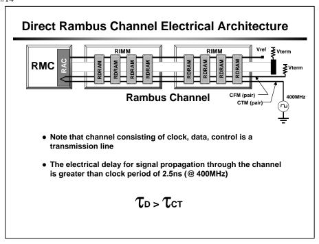
Note that the channel is considered a transmission line because the time that it takes a signal to propagate through the channel is greater than the clock period of 2.5 ns. The propagation time of a signal through the channel is 5-10 ns.
