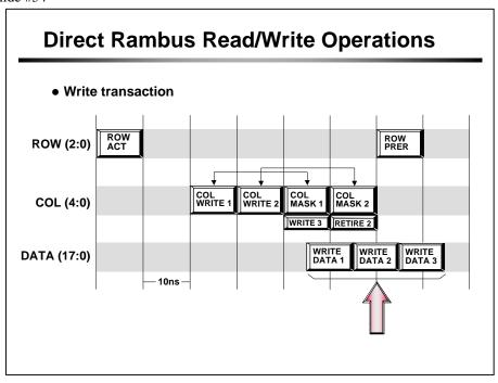
Data is written 6 clocks after the associated COLC packet. But the data is actually written to a write buffer in the RDRAM device first. The write buffer is then retired to sense amps at a later time. The exact time of write buffer retirement is based on a complex set of rules
