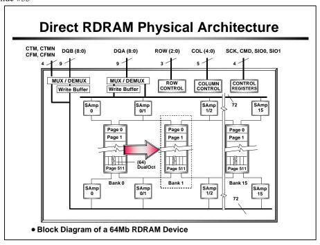
A 64 Mb RDRAM device consists of 16 banks. Each bank contains 512 rows. Thus, each bank holds 0.5 MB of data. A dualoct of data is addressed by specifying the following sub-address:
