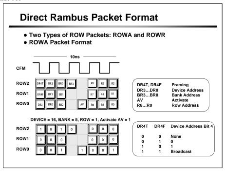
Two types of ROW packets are defined, the ROWA and ROWR packet. The above diagram shows a ROWA (or row activate) packet and the definition of each bit. Like all packets transmitted, the first column of bits of a packet is transferred on the falling edge of CFM clock. Clock and the packet move through the channel together.
