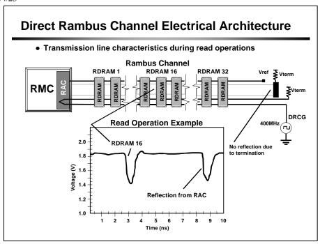
At time t  $\sim$ = 3 ns, the signal reaches RDRAM device 16, meaning that the transmission line delay thus far is about 2.0 ns. Also, at time t $\sim$ =9 ns notice a pulse which is the reflection of the incident wave from the RAC.
