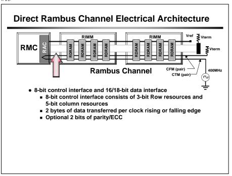
There are a total of 8 Control signals consisting of 3 Row resources and 5 Column resources. The Data bus consists of 2 bytes of data with optional parity/ECC bit per byte.
