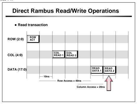
Read Data is available approximately 8 clocks (20ns) after the associated COLC packet. The exact time from COLC before data is returned to RAC depends on:
