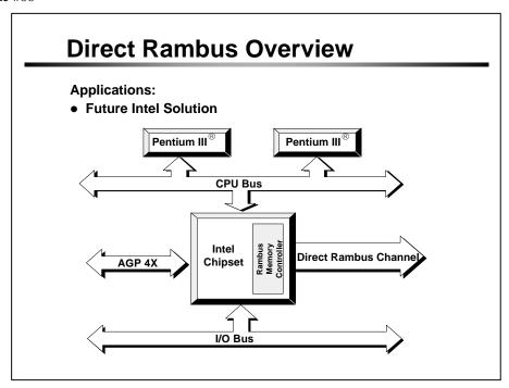
The above picture is a block diagram of a future Intel system architecture. A future Intel chipset will support the Pentium® III processor running at 133 MHz on the host bus. The processor requires a high bandwidth path to main memory. Therefore, Rambus memory architecture is the solution.
