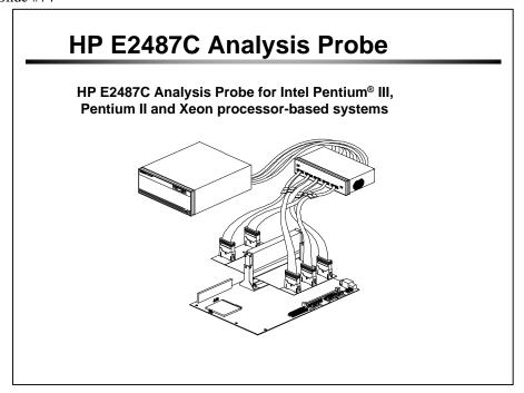
The HP E2487C analysis probe and HP E2492B/C probe adapters are used with the HP 16700A logic analysis system to observe Pentium<sup>®</sup> III, Pentium II and Xeon<sup>TM</sup> processor-based systems. The HP E2487C analysis probe provides a transaction tracker and inverse assembler that can decode Intel processor transactions into bus operation mnemonics. Filter options allow you to selectively list transactions by agent and transaction type.
