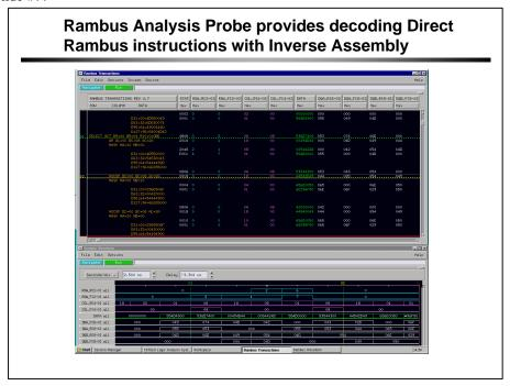
The screen shot above also was taken from an Intel Pentium III processor system. The Direct Rambus analysis probe can show bus transactions displayed in Direct Rambus mnemonics. The top part of the screen has several packs of data that have been decoded by the analysis probe. The Direct Rambus probe captures the data at full channel speed (400 MHz clock speed or 800 MHz data acquisition speed). The bottom part of the screen displays the state data in a waveform format.
