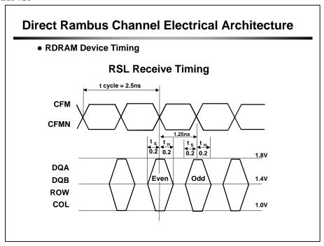
This timing parameter applies to the control signals and data bus during a write transaction. At the RDRAM device, signal setup and hold timing parameters are specified with respect to the falling edge of CFM. The setup and hold parameters are centered around the 0% and 50% points within a cycle time.
