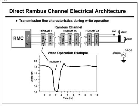
At time t  $\sim$ = 3.0 ns, the signal reaches the first RDRAM device. The transmission line delay is about 1.5 ns at this point.
