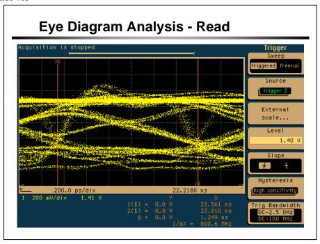
The Direct Rambus read operation is complex and, therefore, more complicated to interpret using eye diagrams. In fact, the only meaningful information that can be obtained from this Rambus line is that it is performing both reads and writes.
