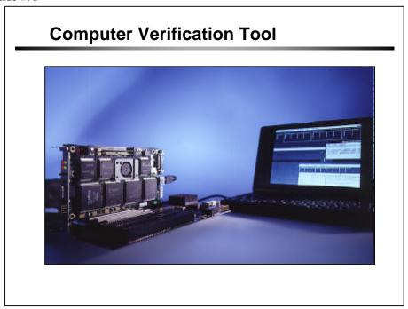
The HP E2920 is the most comprehensive PCI test solution in the industry, encompassing the entire development cycle from bring-up and debug, to I/O system performance characterization, and chip and system validation.
