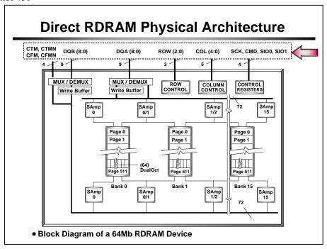
The above figure is a block diagram of a 64 Mb RDRAM device. The arrow points to all the signals present on the RDRAM chip. Their functions have already been described.
