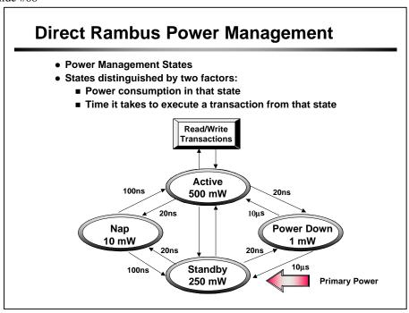
The primary power state of an RDRAM device is the standby state. When in the standby state, the RDRAM device is consuming about 250 mW of power. Whenever an RDRAM device is responding to a transaction, it transitions to the active state. At any point in time, only one RDRAM device is in the active state, unless a broadcast transaction is targeting all RDRAM devices.
