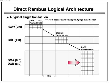
A DATA packets consists of up to 16 bytes of data with 8- or 9-bits per byte. Two bytes of data are transferred per clock rising or falling edge.
