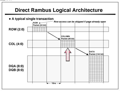
A COL packet transferred by the memory controller is actually split into two fields:
