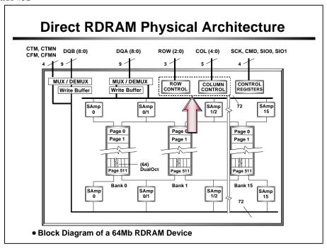
The Row Control and Column Control blocks decode packet information received through the ROW and COL pins.
