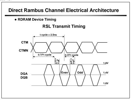
This timing parameter applies to read transactions from the RDRAM device. These timing parameters are specified for the data bus only. Transmit timing is specified with respect to 75% and 25% points within a cycle time from the falling edge of CTM.
