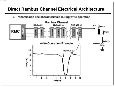
At time t  $\sim$ = 7.0 ns, the signal reaches RDRAM device 32,. Now the transmission line delay thus far is about 5.5 ns.
