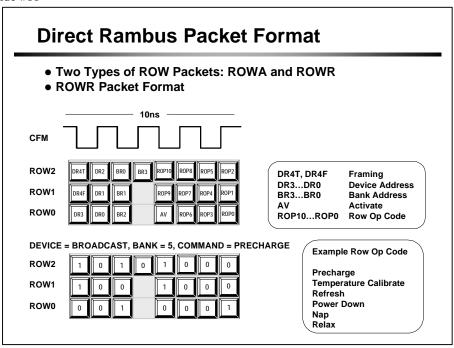
For a ROWR packet, the AV bit = 0. This bit is located at the same position as in a ROWA packet. Also notice that instead of the R bits in the ROWA packet, they are replaced by 11-bit ROP bits. Definition of these bits is shown in the table above. All other bits are self-explanatory.
