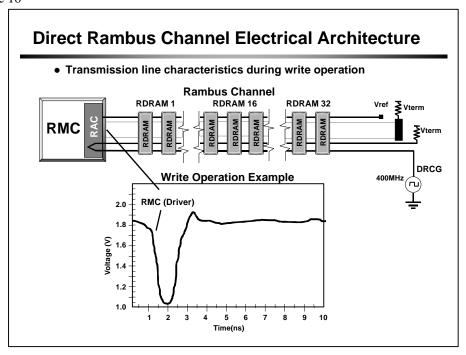
At time  $t \sim 1.5$  ns, the RAC drives the signal low as shown. This signal will propagate down the transmission line
