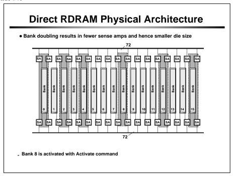
Bank 8 is activated with an Activate row-operation command packet (ROWA) which causes 1 of 512 rows of the selected bank to be loaded into the associated sense amps 7/8 and 8/9.
