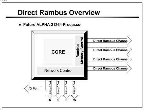
The above block diagram depicts the future 21364 Alpha processor due out in the year 2000. It will run at internal core frequencies greater than 1 GHz. The processor is system memory bandwidth hungry and needs access to large amounts of memory. Rambus system memory architecture is the solution. The processor accesses four channels, resulting in a peak bandwidth of 6.4 GB/s and more than 1 GB memory storage capacity.
