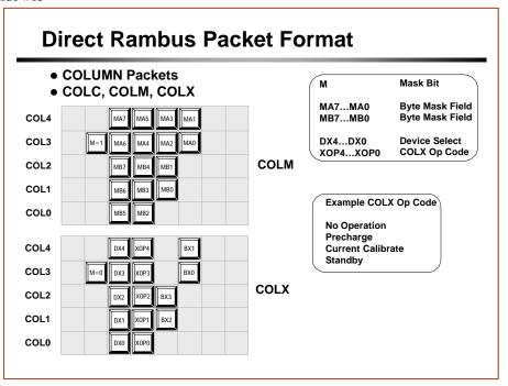
Whenever a Column packet is transmitted it contains a COLC portion as well as either a COLM or COLX portion concatenated. When the M bit = 1, the COLM packet is concatenated, when M bit = 0, the COLX packet is concatenated.
