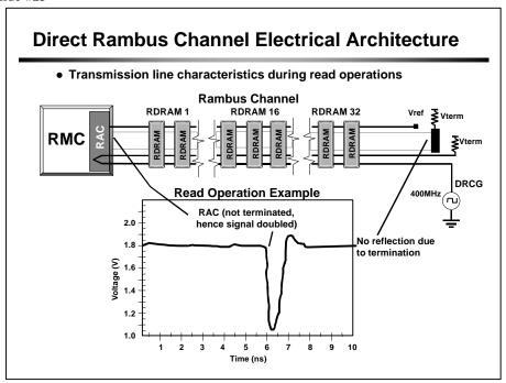
Finally, at time  $t\sim=6.5$  ns, the wave reaches the RAC which has a high input impedance (no termination). Hence the incident wave is reflected and we notice the signal doubling. This voltage transition is detected at the RAC. Note that there are no reflections at the far end of the channel because of termination.
