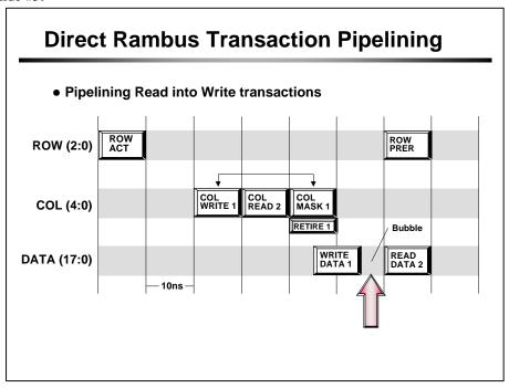
Notice the bubble between write and read data. This bubble exists because of inherent write-read data turn-around time. The data bus is efficiently utilized with the exception of gaps on the data bus that are a result of write operations followed by read operations. Typically, the data bus utilization is greater than 95 %.
