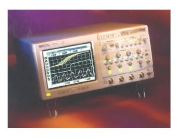
Debugging high-speed bus designs, such as Direct Rambus, often requires a logic analyzer and a high-bandwidth oscilloscope for characterizing the signal integrity of the bus. However, a limitation of high-bandwidth (>2 GHz) oscilloscopes, is that a repetitive signal is needed to take advantage of their measurement capabilities.
