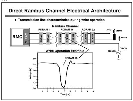
At time t  $\sim$ = 5.0 ns, the signal reaches RDRAM device 16, meaning that the transmission line delay thus far is about 3.5 ns.
