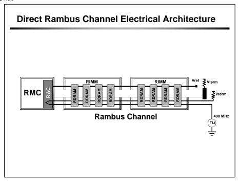
The block diagram above is a representation of a Rambus channel, showing all the components discussed previously, RMC, RAC, RIMM modules, RDRAM devices, DRCG.
