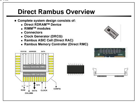
Rambus memory system design consists of the components listed in the slide above.
