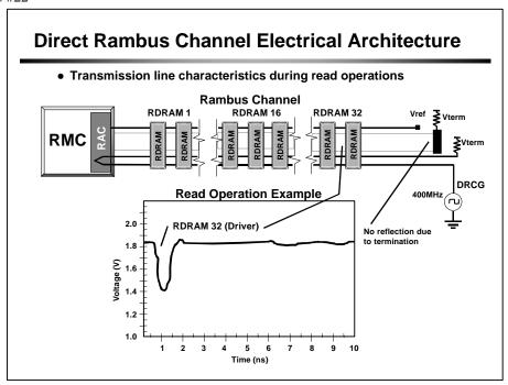
At time t  $\sim$ = 1.0 ns, RDRAM device number 32 drives a logical 1. However, note that the signal is only driven from 1.8 V to 1.4 V. The signal is not driven to 1.0 V. The wave now propagates through the transmission line towards the RAC.
