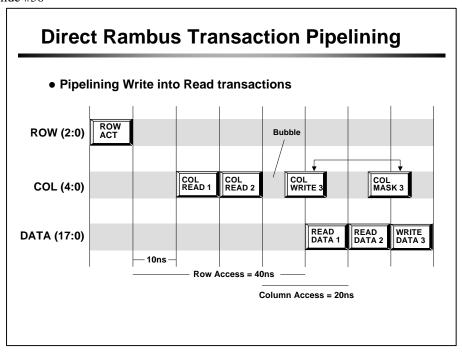
The above diagram shows two back-to-back read transactions followed by a write transaction pipelined into the read transaction. Notice that there are no bubbles on the data bus.
