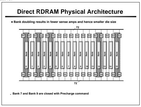
Bank 7 and 9 are precharged with a precharge command, which can be sent either though a row-operation or column-operation command packet.
