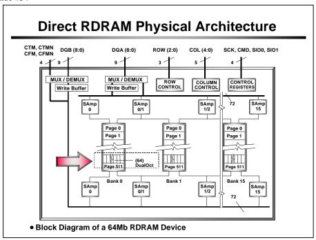
The smallest addressable unit within the RDRAM device is a dualoct. A dualoct is defined as 16 bytes of data. In a 64-Mb device a row shown in the diagram above consists of 64 dualocts (1 KB) of data. This row of information is loaded into sense amps before it can be accessed during read or write operations.
