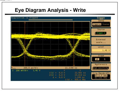
Signal jitter can be measured on a Direct Rambus line by using eye diagram analysis. The above screenshot shows approximately two unit intervals (two bit cells). Common eye diagram measurements include eye height, eye width, crossing %, RMS jitter, and duty cycle distortion.
