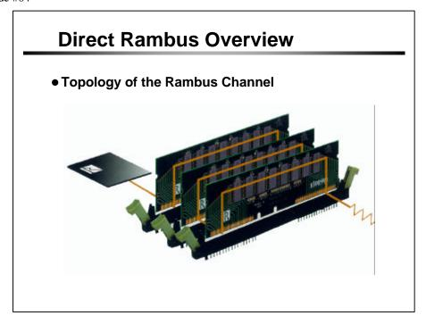
This diagram is a topology view of the Rambus channel showing the memory controller, the connectors, RIMM modules and RDRAM devices. Notice that there are 3 RIMM modules, the maximum allowed. Each RIMM can have up to 16 RDRAM devices, but a maximum of 32 devices are supported per channel.
