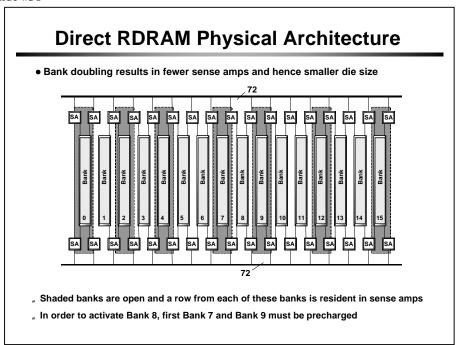
This example demonstrates the concept of bank doubling. The shaded banks are open or activated and a row from each of the shaded banks is contained in adjacent sense amps.
