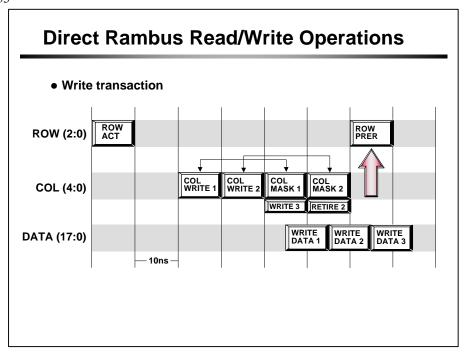
This row precharge packet (ROWR) is used to precharge the open row, which was activated a little earlier by the ROWR packet shown. The ROWR packet contents include:
