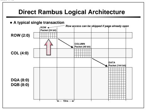
The transaction protocol supports two types of ROW packets transferred by the memory controller:
