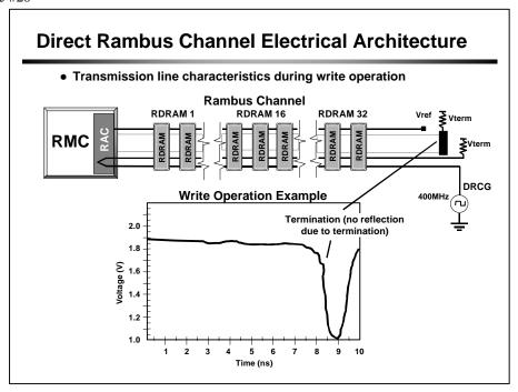
Finally, at time  $t \sim 9.0$  ns, the signal reaches the end of the transmission line and the termination point. There is no reflection at this point. The transmission line delay thus far is about 7.5 ns.
