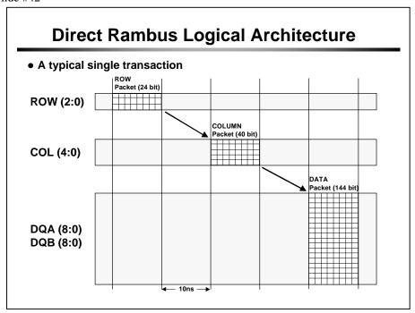
A typical read or write operation initiated by the memory controller consists of the transmission of a ROW packet followed by the transmission of a COL packet. If the operation is a write operation, then the memory controller also sends a DATA packet. If the operation is a read operation, the DATA packet is transferred by the RDRAM device that is being read.
