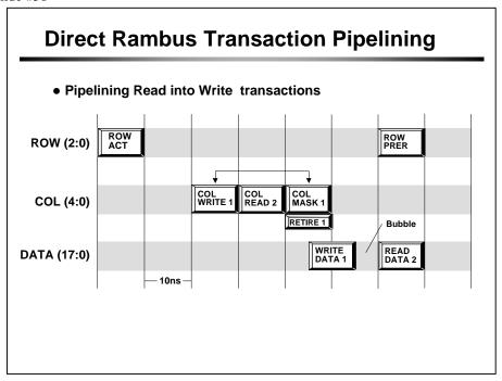
The above diagram shows a write transaction followed by a back-to-back read transaction. Notice that there is no bubble inserted by the memory controller on the COL bus.
