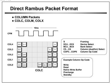
Now, let's look at COL packets. The above diagram shows the COLC portion of the COL packet. A valid COLC packet contains the S bit = 1. The 4-bit COP field indicates the kind of column operation being initiated, such as, read or write etc. The 6-bit Column Address (C) field points to the exact dualoct (1 of 64) within the row contained in the sense amps that are being accessed.
