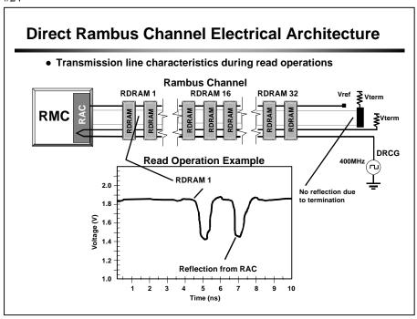
At time  $t \sim 5$  ns, the signal reaches RDRAM device 1, meaning that the transmission line delay thus far is about 4.0 ns. Also, at time  $t \sim 7$  ns notice a pulse which is the reflection of the incident wave from the RAC.
