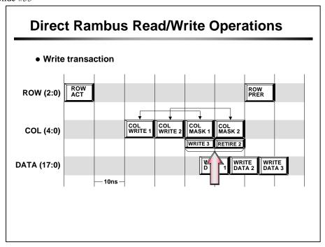
The first COLC packet, indicated by the arrow in the slide above, is the third write packet in this diagram. This COLC packet will cause the write buffer to retire of the first data packet written. Concatenated to this packet is a COLM packet. The COLM portion of this COL packet is associated with the previous COLC packet, 8 clocks earlier. The COLM packet specifies Byte Masks for the dualoct data to be written.
