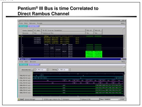
The screen shot above was taken from an Intel Pentium III processor system and displays time-correlated data from the CPU 0 bus to the Direct Rambus channel.
