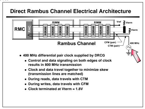
The DRCG at the far end of the channel supplies the 400 MHz differential clock pair. Control and data signals are clocked on both edges of the clock resulting in an 800 MHz effective transfer. Clock and data travel together. Therefore, the skew between clock and data is kept to a minimum (< 100 ps). If the clock and data do not travel together, it is not possible to meet setup and hold times at this high of a frequency.
