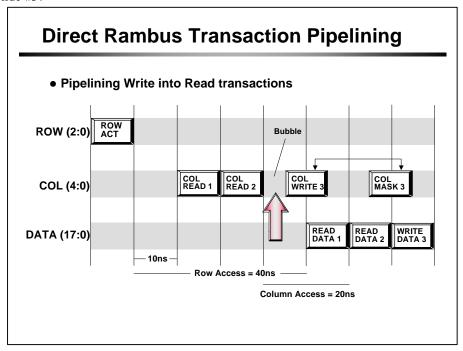
Notice the bubble between read and write COLC packet which is inserted by the memory controller. This bubble is needed to delay the write data until the read data from the previous read has arrived at the memory controller. The data bus is efficiently utilized.
