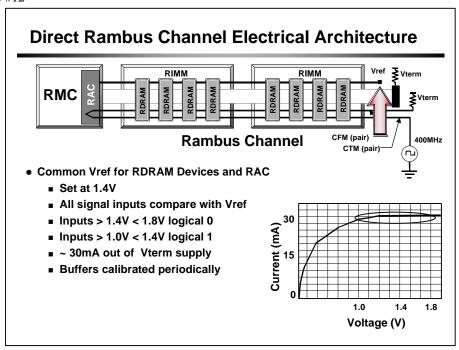
RSL signal swing is uniform around 1.4  $V_{ref}$ .  $V_{ref}$  is an input to all devices on the channel. When an RSL signal is asserted (1.0 V) the driver sinks ~ 30 mA of current. This current is uniform across RSL signaling levels as shown in the graph above. The drivers are current calibrated periodically as explained later in the presentation to ensure that the signal swing remains uniform over time.
